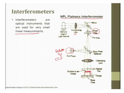
Interferometer are optical instruments that are used for very small linear measurements. So, you have this is an NPL flat interferometer mercury vapour is there or you can put a laser there, a condenser lens is there. So, you have a mirror, then you put green filter, then you have pinholes through which the light passes through, then you have a glass plate reflector, you have an eye piece here.
