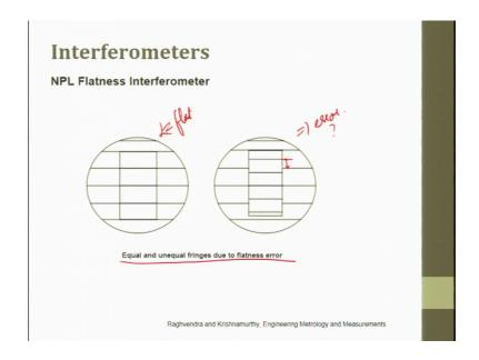
So, if the surface is flat, you can see the fringe patterns continuously are the same. If there is a difference in flatness, then you can see there is a shift in the fringe patterns which is done. So, equal and unequal fringe patterns due to flatness error, this is a flat surface, this is a error surface. So now, you can see that distance whatever it is and then you can the number of fringes distance what you measure, you can try to find out what is the error.
