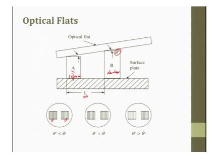
So, these are the 2 slip gauges. So, you can see a can be a reference. This can be maybe what you have developed. So, this both has to be kept on a flat one, this is the distance called L, and this is the small degree and the flat which is placed at a small degree theta. So, when if both theta dash and theta are same you will see the same fringe patterns.
