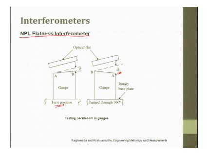
So, the NPL flatness interferometer works like this; the gauge is there. So, you have 2 surfaces, the formula is the same. So, it is placed at an angle. So, you try to take the first position, then you turn it around the gauge and then rotate the table, then place the gauge B A and try to measure the delta 2, using the same optical flat. If you see both the fringe patterns are the same, then these two are flat surfaces.
