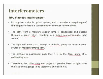
It comprises a simple optical system which provides a sharp image of the fringes so that it is convenient for the user to view them. The light from the mercury lamp is condensed and passed through a green filter resulting in the green monochromatic light source; the light will now pass through a pinhole giving an intensity point source for monochromatic light.
