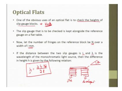
One of the obvious use of optical flat is to check the height of a slip gauge Block. We studied the slip gauge for end measurement. So, we could we made blocks on slip gauge, and these blocks for measuring height we used.
