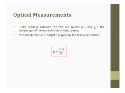
So, if the distance between the 2 slip gauges L and lambda and L is the wavelength of the monochromatic source, then the height difference h is given in the following relationship.
