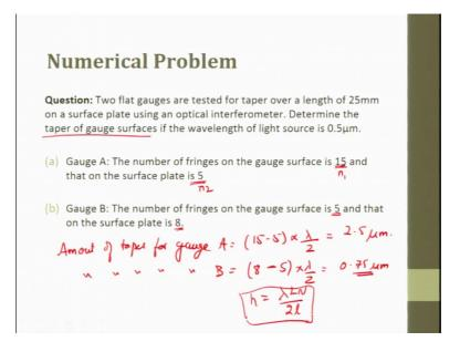
So, let us try to solve another problem and see the 2 optical flats are tested for taper over a length of 25 millimeter on a flat plate using an optical interferometer. Determine the taper of the gauge surface if the wavelength of the light sources 0.5. Gauge A the number of fringes on the gauge surface is 15, and that on the surface plate is 5. Gauge B the number of fringes on the gauge surface is 5 and that on the surface plate is 8.
