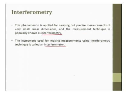
This phenomena is applied to carry out precise measurement of very small linear dimensions and the measurement techniques is popularly known as interferometry. The instrument which is used for measurement is called as interfero meter.
