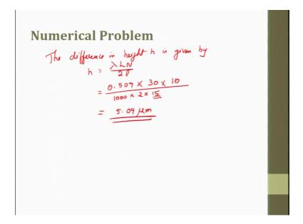
So, the difference in height h is given by the formula; is given by h equal to lambda L N by 2 l. So, this is lambda is 0.509 and what is L? L is 30, what is L? L is the distance between the 2 blocks is 30 into n which is said to be in 10 millimeter it is this much.
