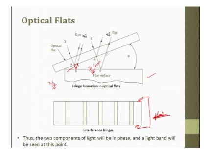
So, next one is optical flat. This is the optical flat, optical flat means you have an optical optical glass, assume it as a plate. The top surface and the bottom surface is completely made flat. And this is predominantly used for generating fringe patterns.
