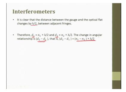
So, it is clear the distance between the gauge and the optical flat changes by lambda 2 by adjusting fringes therefore, d 1 is given as n 1 lambda by 2 d 2 is given as n 2. So, d 2 minus d 1 is this, which we already seen. So, by this relationship is used to measure the flatness error on the surface.
