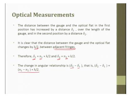
So, the other optical measurements are the distance between the gauge, and the optical flat in the first portion has increased by a distance lambda 1 dou delta 1 over the length of the gauge, and in the second position by a distance of lambda 2
