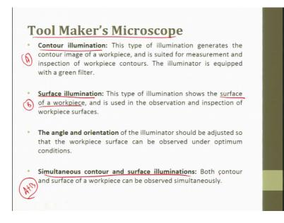
So, these are the different types of illumination, you can have and more details about the tool maker's microscope. Contour illumination can be done, this type of illumination generates the contour image of the work piece and is suited for measurement and inspection of work piece contour, the illuminator is equipped with a green filter. So, now that you can also try to place you know I have said 3 basic parameters, one is wavelength amplitude and then you have the polarization.
