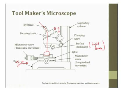
So, this is a typical tool maker's microscope. So, this is the column which tries to take the load.
