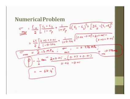
So, sigma max the formula goes like E m by 2 strain 1 plus strain 3 1 minus poisons ratio plus 1 by 1 plus poisons ratio root of strain 1 minus strain 3 the whole square plus 2 times strain 2 minus strain 1 strain 3 the whole square. So, this is for sigma max. So, sigma max with you substitute all the all the things.
