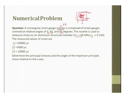
So now, let us try to work a simple problem a rectangular strain gauge rosette. So, rosette is it looks something like you have this way and this way will be at an angle. So, 2 directions a rectangle rosette is composing of strain gauges it will. In fact, rosette is for 3 directions right. So, oriented at relative angle 0, 45 and 90 degree. So, you will have 3 types of strain gauges, in uniaxial you had only 1. So, this 3 strain gauges are located at 0 45 and 90 degrees.
