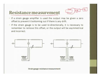
So, if a strain gauge amplifier is used to. So, where is a strain gauge amplifier coming? So, you have a member then you stick strain gauges to the member you track and output from the strain gauge. So, it is attached to an amplifier from that amplifier. It will be shown as a output display whatever it is. So, if the strain gauge amplifier is used is used, the output may be given a 0 offset to prevent it bottoming out if there is a drift.
