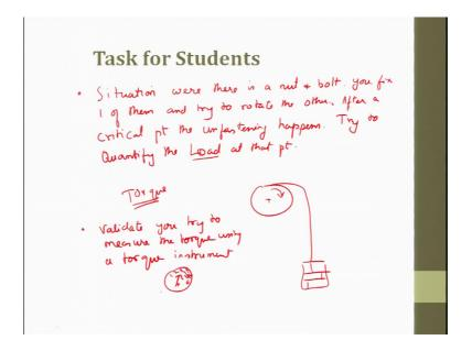
So, task for the student try to take a situation where there is a nut and bolt, you fix one of them and try to rotate the other ok. And after a critical point, the unfastening happens try to quantify the load at that point.
