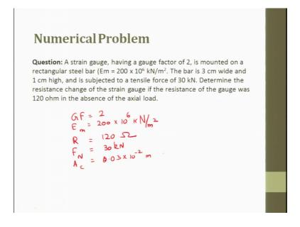
Now, let us see a simple problem a having a gauge factor of 2 is mounted on a rectangular steel bar the bar is 3-centimeter-wide and 1-centimeter-high and is subjected to a tensile force of 30 kiloNewton. So, determine the resistance of change in the strain gauge if the resistance of the gauge was written 20 ohms in the absence of axial load.
