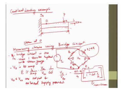
So, now let us see how do we stick it on top of a beam which is getting loaded or beam loading example, we can see or beam load or transverse load or axial load taking. So, the beam is attached to a, this is a fixed end, this is the cantilever ok. So, here the length of
