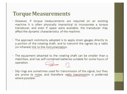
However, if the torque measurements are required on an existing machine, it is often physically impractical to incorporate a torque transducer and even if space where available. The transducer may affect the dynamic characteristics of the machine. So, for an existing machine, torque measurement is slightly difficult. So, we have to make keep that in mind for a developing one. When there are in part wise and subassembly wise, yes, you can do.
