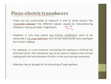
They can be constructed to measure in 1 2 3 planes 1 2 3 planes the cross talking between the different planes caused by manufacturing limitation being normally insignificant. So, you have extraction y direction and z direction y x and z. So, you stick strain gauges in all the 3 directions. So, once response will not be communicated to the second one. So, that is called as cross talking.
