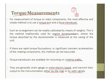
Next one is torque measurement. Torque is nothing but a rotational when there is a member and in this number is fixed at one end and you try to rotate the other end, in the clockwise or anticlockwise direction, what load comes as a torsional load for measurement of torsion or a and static component the most effective and the simple method is to used the torque arm and the force transducer.
