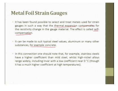
It has been found possible to select and treat metals used for strain gauge in such a way that the thermal expansion is compensates for the resistivity change in the gauge material. So, this effect is called as self-compensation. They compensate for the thermal change.
