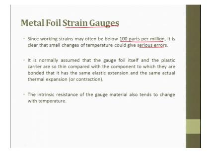
Since working strain may often be below 100 parts per million, it is clear that small changes of temperature could be very serious error. So, please make sure, when we use the strain gauge measurement the temperatures are not dominating. It is normally assumed that the gauge foil itself and the plastic career are. So, thin compared with the component to which they are bonded that, it has a small elastic extension and same actual thermal expansion.
