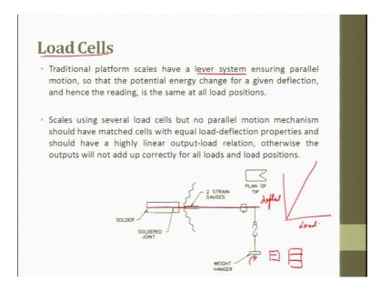
Now, let us see the next thing which is called as load cell. Traditionally, platforms scales have a lever system ensuring parallel motions. So, that the potential energy change for a given deflection and hence the reading is the same at all load positions for example, this is traditional one scales have a lever system ensuring parallel motions.
