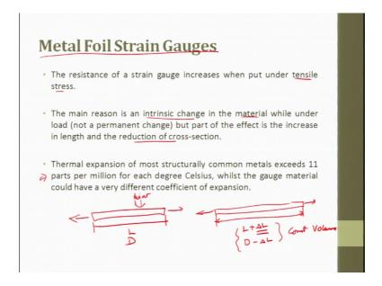
So, load cell is 1, the next one is the metal foil strain gauges the resistance of a strain gauge increases, when put tensile stress tensile compression, but predominantly we used for tensile stress.
