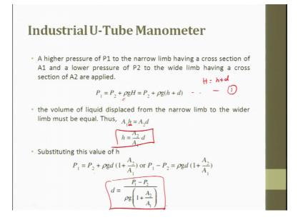
The higher pressure of P 1 to the narrow limb have a cross section area of A 1 and a lower pressure P 2 to a wider limb having a cross section area of A 2 is applied. So, P 1 equal to P 2 plus rho g H; where this heads if you go back to the figure and see it is H is equal to small h plus d.
