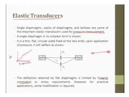
The next type is going to be a transducer, so, basically a transducer is we studied transducers in detail. So, elastic transducers this is nothing but you have a diaphragm, a single diaphragm stack of diaphragm single diaphragm can be there, a stack of diaphragm can be there, the bellows are some of the important elastic transducer used for pressure.
