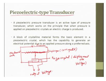
Next one is piezo type transducer, the piezo type transducer so; here what will happen is you will have a piezo crystal from which you take outputs. So, this is the output voltage and this is a piezo crystal ok. So, this in turn is attached to a diaphragm so, this is your diaphragm if you want to increase sensitivity you can make it corrugated.
