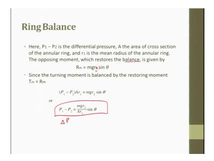
So, here P 1 minus P 2 is the differential pressure. A is the area of cross section of the annular ring, r is a mean radius of the annular ring. The opposing moment so, here what we are trying to do is turning moment T m is equal to this.
