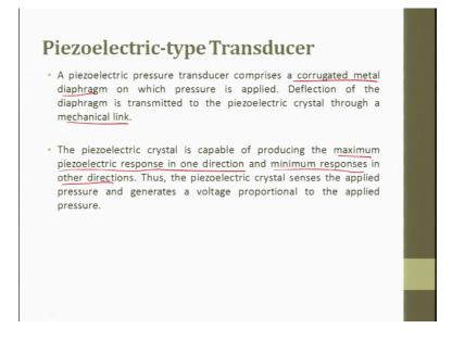
So, as I told you the transducer comprises of a corrugated metal diaphragm on which the pressure is applied. So, there is a mechanical link to attach it with the sealing and it the piezo crystal is capable of producing the maximum piezo response in one direction and minimum response in the other direction. Thus, the piezo crystal senses the applied pressure and generates a voltage proportional to the applied pressure so, this is what is a diagram we saw here.
