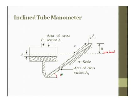
So, this is an inclined type tube type manometer. So, I here you have a 0 line this is called a zero level h d this is a scale here and here is the inclination which is there and this is the angle theta. Suppose here you want to find out what is d so, what is pressure difference P 1 minus P 2 it is rho into g into x sin theta.
