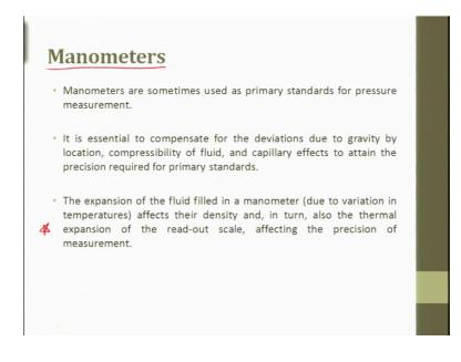
So, to measure we pressure we thought or a very primitive device for measuring pressure is a manometer. Manometer are sometimes used as a primary standard for pressure measurement, it is a very, very basic thing. It is essentially to compensate for the deviations due to gravity by location compressibility of fluid, capillary effect to attain the precision requirement for a primary standard ok.
