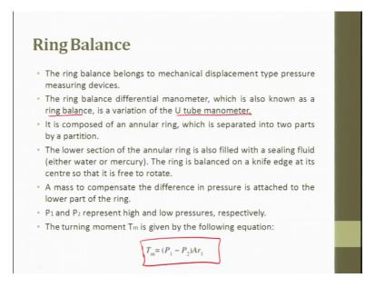
So, next one is ring balance, a ring balance belongs to a mechanical displacement type pressure measuring device. The ring balance differential manometer which is also known as ring balance is a variation of U-tube manometer. It is composed of an annular ring,
