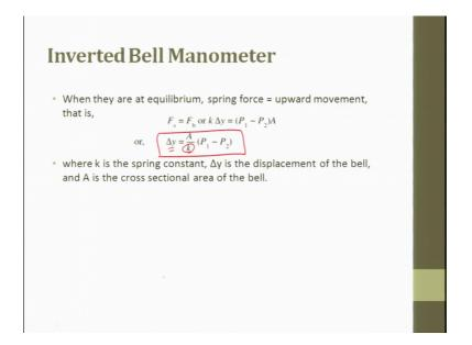
So, when they are at equilibrium it is F s equal to F b or it is stiffness into delta y which is nothing but P 1 minus P 2 into A. So, this delta y can be represented as A by k P 1 minus P 2, k is the spring constant and delta y is the displacement of the bell and A is the cross section area of the bell. It is another type of manometer which is used to measure the pressure, but the most important point is it is capable of measuring absolute, positive, negative and differential pressure.
