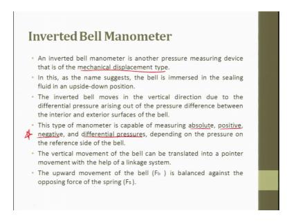
So, let us see the explanation, an inverted manometer is an another pressure measuring device that is of mechanical displacement type. This type as the name suggested the bell
