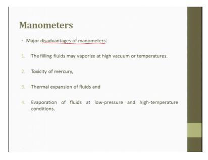
The main disadvantage of manometer is the filling fluid may vaporize at high vacuum or temperature. The filling fluid may vaporize at high vacuum or temperature. Toxicity of mercury is very very important point where mercury if it starts vaporizing. Thermal expansion of the fluid and evaporation of the fluid at low pressure and high temperature conditions, these are some of the very important points which makes difficulty in using manometer.
