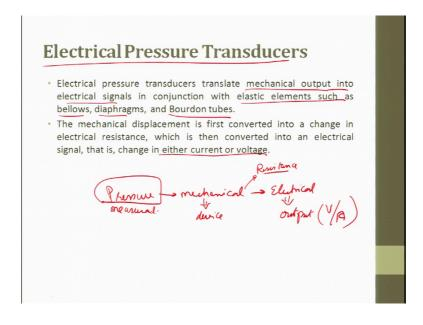
The electrical pressure transducer is the latest one which is coming up here. The electric pressure transducer translates mechanical output into an electrical signal in conjunction with the elastic elements such as bellows, diaphragms and bourdons. So, basically what we wanted is the pressure is to be measured they measure it in a mechanical means and then this mechanical values are converted into electrical value so that it can be processed for further action.
