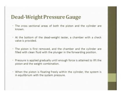
The cross section area of both the piston and cylinder are known. The bottom of the dead weight tester chamber with a check valve is provided. The piston is first removed and the chamber and the cylinder are filled with clean fluid with the plunger in the forward position. The pressure is applied gradually until enough force is attained to lift the piston
