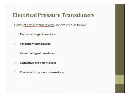
The electric pressure gauge are classified as follows; that is resistance type transducer, potentiometric device, inductive type transducers capacitive type transducers and piezoelectric pressure transducers. These are some of the electric pressure transducers which are available in the market today.
