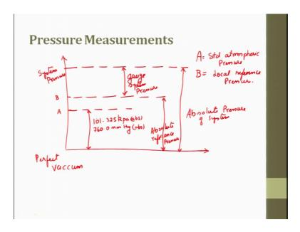
So, let us just put this in diagram. So, this is perfect vacuum, this is system pressure, this is I am write it as A and then I will write it as B; that A is nothing but standard atmospheric pressure and B is nothing but local reference pressure. This one is called as absolute pressure of a system pressure of a system, this one is called absolute reference pressure. The difference between these two are called as gauge system pressure.
