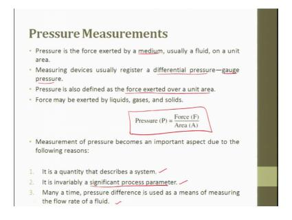
Pressure measurement, pressure is force exerted by a media usually a fluid or a unit area. Measuring devices usually resist a differential pressure for example, gauge pressure we will see what is gauge pressure later. That does not need the pressure is also defined as force exerted over a unit area, pressure may be exerted by liquid, gas or solid. So, this is the definition for pressure, pressure is nothing but force acted per unit area.
