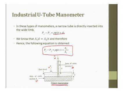
In this type of manometer a narrow tube is directly inserted into a wide tube. So, this is a second type so, this one we can try to find out d. So, we will look for another industrial U-tube manometer, which is called as cisterns manometer. So, almost the same thing can be done here so, what we do here is, we take a cylinder fill it up with liquid and then we
