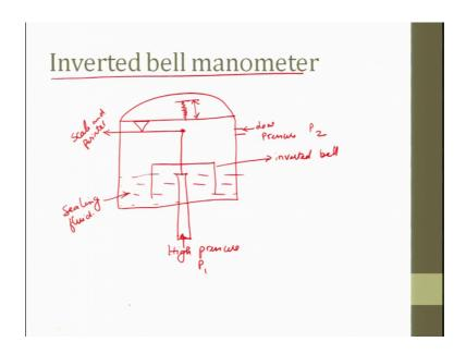
So, the next type manometer is going to be inverted bell type manometer. So, let me draw the figure of a inverted bell type manometer. So, this is a low pressure low pressure P 2, this is high pressure high pressure high pressure P 1 ok. This is a sealed sealing fluid, this is a pointer scale or a pointer scale and pointer ok. And this is the inverted bell, this is a inverted bell. So, this is how a inverted bell manometer looks like.
