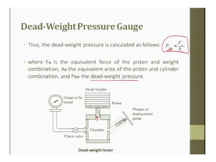
So, if you look at it this is like this so, here is a pressure gauge so, here is a chamber a dead weight is there. So, a plunger or a displacement pump is there so, here so, this weight is balanced and we try to measure the gauge it works on Archimedes principle.
