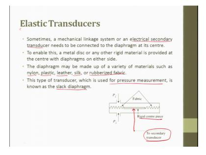
So, elastic transducer sometimes a mechanical linkage system or an mechanical linkage system. So, you can see pressure springs are applied mechanical linkage system, or an electrical secondary transducer need to be connected to the diaphragm at the centre. So, this is a secondary transducer which is connected to the centre. So, this enables a metal disc or a rigid material is provided at the centre with diaphragm on either sides.
