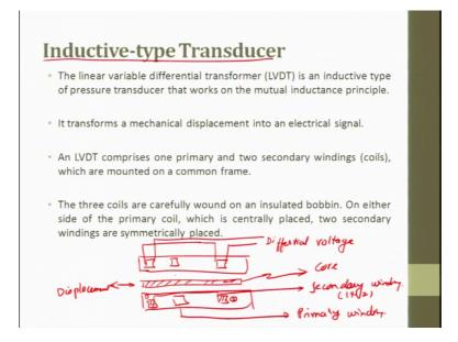
So, the next one is inductive type transducer which is the other which is otherwise called as a linear variable transducer LVDT. So, here what happens is like we saw in the previous slides also, you have two things. And in between you have a core, this is called the core ok and here you will have primary winding and you will have secondary winding. So, you can call this as primary winding, this and this are called as secondary winding ok.
