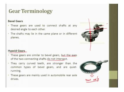
This is a bevel gear. So, bevel gear look at it so, here is an axis here is an axis right. These gears are usually to connect shafts at an desired angle to each other. So, here I have just put perpendicular, but if you see more closely this is certain angle, this is certain angle, but here I have just intentionally draw it as 90 degrees.
