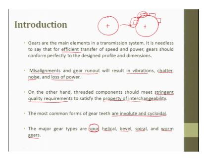
Gears are the main element in transmission system. As, I said from one point to another point you have to transmit power. So, then gear is one of the main element which is used for it. It is needless to say that the efficient transfer of speed and power gear should confirm perfectly to the designed profile and dimensions.
