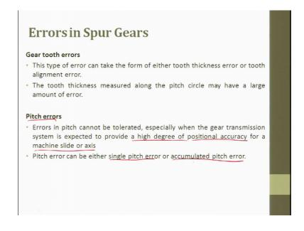
Then gear tooth error, this type of error can take the form of either tooth thickness error or tooth alignment error, tooth single teeth, the single geometry in a gear is called as the tooth several tooth put together makes a teeth gear teeth. The tooth thickness measured along the pitch circle may have a large amount of error.
