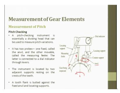
Then, the other check we have this pitch checking, a pitch checking instrument is essentially a dividing head dial gauge it has a dividing head that can be used to measure pitch variation. So, here you will have a measuring feeler and then here you will have a locating pin which is a pin, which locates the gear being inspector it locates here. So, then every time what we do if we try to index, when with this index we try to take gear after gear after gear we try to check the pitch.
