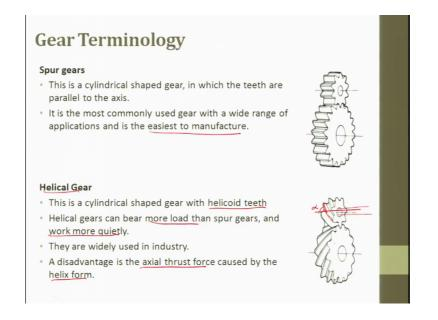
When, we talk about spur gear this is a typical spur gear. This is a cylindrical shaped gear, in which the teeths are parallel to the axis. This is the axis, teeths are running parallel to the axis. This is the most commonly used gear with a wide range of application and it is easiest to manufacture. Lot of gear trains use spur gears right. So, this is the most common gear and lot of inter changeability concept can be followed in these gears.
