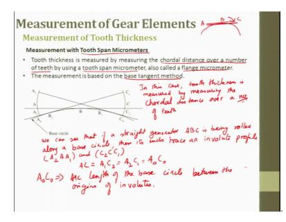
Till now what we were doing is we were measuring it for a single teeth. Now, we will try to measure for a set of teeth. So, for which we use tooth span micrometre. Till now we have did only one tooth, now will take some 3 4 tooth and then try to measure tooth thickness is measured by measuring the chordal distance over a number of teeth by using the tooth span micrometre also called as flange micrometre.
