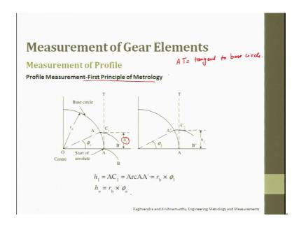
So, measurement of gear element so, we wanted to measure the gear profile. So, we want to measure it by using the first principles of metrology. So, in this figure let us first try to understand. So, this is the base circle, this is the base circle the radius of the base circle is going to be r b right.
