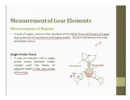
So, what are the different ways of measuring the gear elements? So, first we are trying to measure the run out. So, in case of gear run out is a resultant of a radial through of the axis of a gear due to out of roundness of the gear profile. So, there is a centre. So, there is a shift in the centre. So, a radial throw of the axis of a gear, due to the out of roundness of a gear profile, the run out tolerance is the total allowable run out.
