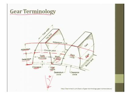
So, if we start looking at Gear Terminology. So, the first thing which you should understand is the pitch circle, pitch circle is this which passes through which is almost in the mid of the tooth is pitch circle. Top of the pitch circle up to the face of the teeth, if you try to draw one so, that circle is called as addendum circle. So, this is a pitch circle which a circle which passes through the face, top tooth face right or the yeah tooth face. So, that is called as addendum.
