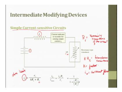
Next we will move into simple current sensitive circuits. So, here we see that this is the applied energy input energy this is the resistance R to the suffix r, then the current indicator or recorder of sensing output of current i naught, then you have R t, which is resistance type transducer where k is the magnitude which or a factor which can be multiplied with the current in term the i naught is expressed in terms of ei by k R t by R r by R suffix r
