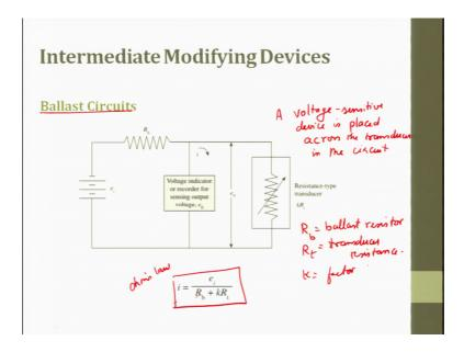
So, the next one is going to be Ballast, Ballast circuit. So, here we will have e i which is an applied voltage. So, this basically this is a small variation here a voltage here a voltage sensitive device is placed across the transducer across the transducer in the circuit this is small variation to the simple circuit. So, it is placed here. So, that we try to get the current variation. So, it is important to note that that in the absence of R b.
