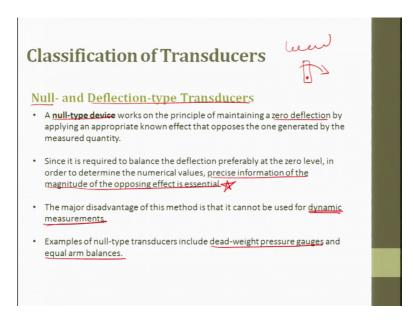
Then you have null and deflection type transducer we saw this null in comparators. So, you can also have a null type device working on the principle of maintaining a 0 deflection by applying an appropriate known effect that opposes the one generated by the measured quantity. So, it is always in 0; or you try to put a measured value. So, then it immediately shows the displacement and from the displacement, you try to apply some force and bring it to 0.
