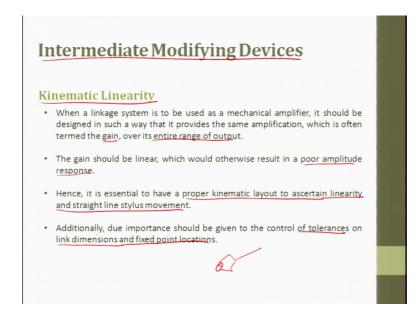
So, now we have seen the primary part now we will move to the next part which is the intermediate modifying device. So, here kinematic linearity is very important when a linkage system is to be used as a mechanical amplifier, it should be designed in such a way that it provides the small amplification which is often termed as gain over its entire range of output ok.
