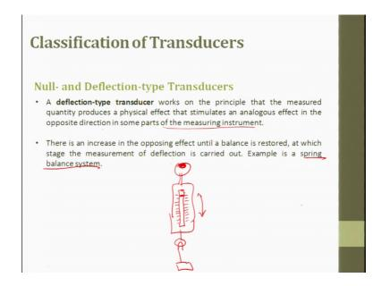
So, the deflection type transducer works on the principle that a measured quantity produced a physical effect that stimulates an analogous effect in the opposite direction in some part of the measuring instrument I repeat works on the principle that the measured quantity produces a physical effect measured quantity is displacement quantity produces
