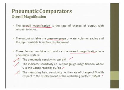
Now, if we want to look at the overall magnification, the overall magnification is the rate of change of output with respect to input that is magnification. The output variable in the pressure gauge or water column reading today it is only pressure gauge and the input variable is surface displace is a surface displacement.
