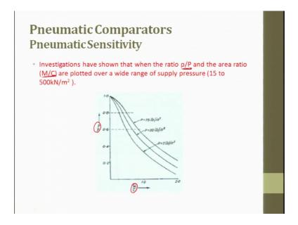
So, the sensitivity of a pneumatic gage can be brought like this. So, this is dp by p and this is M by C. So, there is a ratio. So, we try to put these two in ratios and then we try to take a linear range whichever is there and try to operate our device within that linear range.
