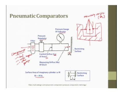
What happens in a numerical comparator or pneumatic comparator how does the circuit look like? Basically, what happens you try to take air from a compressor. So, whenever you try to take an air through a compressor what you do is you try to take free air, then you try to compress the air, when you try to compress a free air there is a possibility that you might have dust, you might have some amount of water vapor and you might have other foreign particles.
