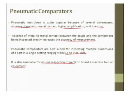
Pneumatic metrology is quite popular because of several advantages it has absence of metal to metal contact. So, there is no wear and tear high amplification can be done depending upon your circuit, pneumatic circuit what you develop and it is low cost reliable
