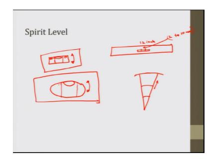
So, if I draw this as my sprit level this is 12 inch, and this voile the distance between the 2 lines, you can see the 2 markings are there, 2 black lines are there on the voile. You can see closely that there 2 black lines ok. The bubble has to remain within this black lines, there is not has to be any parallax error. So, let me make it very parallel to the camera ok. Now you can see the bubble is exactly in the 2 lines ok.
