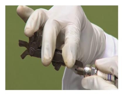
So, let us try 1 mm. It is looks like a good fit; it is fitted properly. To confirm it we will use the rule of go and no go gauges. So, it I think it is 1 mm, that pitch of this screw of this spark plug is 1 mm only. I will confirm it by using 0.9 mm also.
