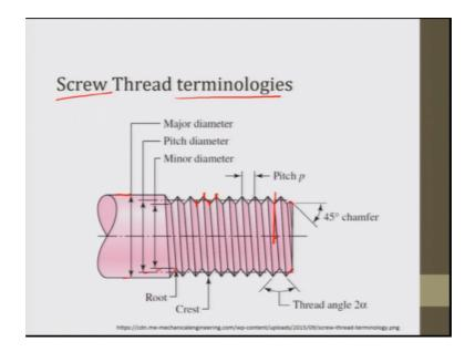
So, let us recall this screw thread terminology before I show you the actually tool here. So, this is the screw thread terminology. Here we have the major dia, the minor dia, the minimum dia and we have pitch diameter ok. So, there is root and crest, we have trough and crest.
