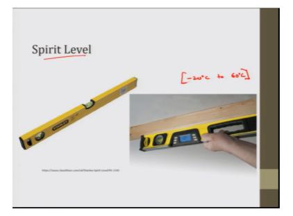
So, next instrument I will pick here is spirit level. Spirit level is an instrument or else it is a simple level or an instrument that is used to see whether a surfaces are horizontal or vertical, or is there any difference in the level or not; which is used by carpenters, masons or the for checking the bricklayer brick line, that is the wall getting straighten or not, we can you might have seen that. And in mechanical metrological lab it is also used sometimes.
