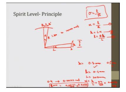
So, I can explain this using the principle of the spirit level here. So, what happens? If my bubble is here, this is my bubble ok. It changes it is position from B to B dash, and this changing position this length is 1. And the radius of the voile is let me say R, this is center the radius is R. This angle is the angle that the 2 ends of the bubble 2 ends of the line make with the center of the circle. I call this angle as alpha.
