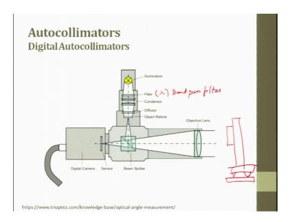
So, digital when you look at digital autocollimator you see that there is an objective lens then there is a beam splitter, beam splitter is there for both. Then this beam splitter goes to an objective reticles then diffuser condenser to condense this and then you have filters. This filters can be more or less you can decide what filter to use and you can decide what
