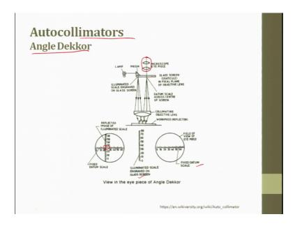
So, this is an auto dekkor, so you have lamp this is a prism. So, have a microscope from here the light goes hits at a collimator and this is the collimating and this is an objective lens, here is the work piece surface it reflects back and then we have a glass screen which is in the focal plane of the objective lens we have. So, from here we try to see through the eyepiece and try to get the data.
