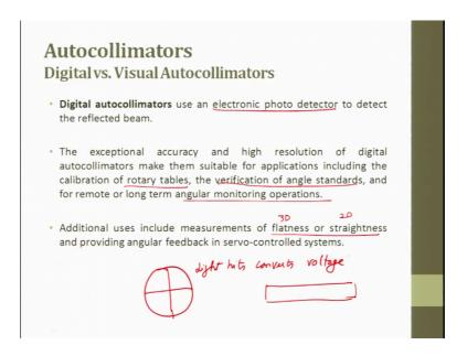
Autocollimator is a device where in which we used light this light will be hitting at a mirror, this mirror will be placed on a surface where you want to do measurement. Based upon the reflection we capture it back and then we try to figure out from the inference pattern or from the shift in cross section or cross wire we try to find out the shift from that we try to calibrate the angular deviation which is on a surface.
