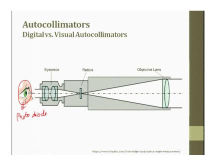
So, this is how we test, so here is the objective lens this is the eyepiece and you have reticles here, so here is an operator the operator eye is otherwise converted in a digital form it is converted into a photodiode, so it is a photodiode.
