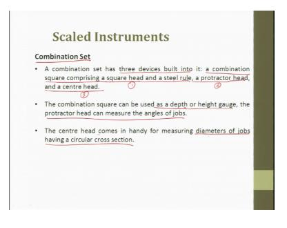
Next one is an interesting thing which is a combined set. A combined set has three devices built into it. So, till now what we saw was only a single instrument a V block right; a V block, a flat plate a depth gauge, maybe a Vernier or screw gauge.
