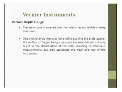
You also have Vernier depth gauge; Vernier depth gauge is a more versatile instrument which can be used for measuring up to this smaller. The lower surface of the base has a blunt form lay against the upper scale of the hole and recess. So, it we have already discussed. So, it has a nut to slide and then loosen it. The main scale is lower and then one should avoid excessive force to be applied. So, that it does not deflect.
