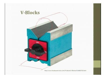
This is a V block. So, here in this V block, we always try to put a cylindrical piece, a cylindrical piece is put and then if you want to measure the height of it you can start measuring it. If it is a magnetic material, so all you have to do is you put a flat plate and then you try to rotate the knob and magnetize it such that this V block gets firmly fastened to the surface plate whatever you have, it is because of the magnet present. So,
