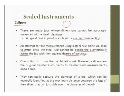
The next one is a caliper, a caliper is basically to take the dimensions but it will not give you the values. It is only to take the dimension, take the shape and then transfer it. So, there are many jobs whose dimensions cannot be accurately measured with steel ruler alone.
