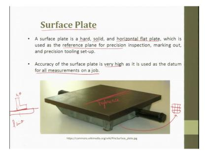
So, this is an instrument which is called surface plate. Surface plate are generally made out of hard is a hard solid horizontal flat plate, which is used as a reference plane for precision instrument. See what happens when you start the doing all these measurements. At least one datum one datum should be flat or one datum should be reference.
