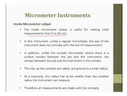
So, here is that lease count which is displayed which talks about 1 micrometer. Inside micrometer, so, inside micrometer the inside micrometer is used for making very small measurements from 5 to 25 millimeter.
