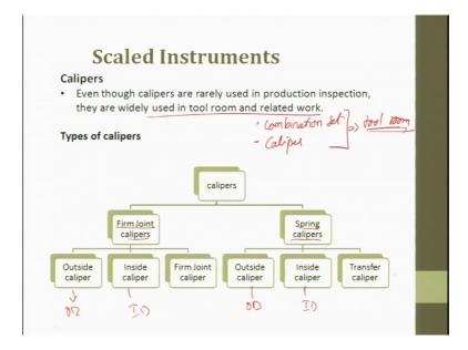
So, even though calipers are rarely used in the production inspection, they are very widely used in the tool room. So, combinational set combination set is also operation is very difficult combinational set then we talk about caliper, these are all used in tool rooms. Tool room basically tool rooms are rooms where in which is used for grinding or manufacturing a tool which can be used in the regular process line or they try to make tools.
