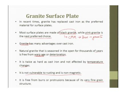
So, granite surface plate; granite surface plate I have started replacing cast iron surface plates. Most surface plates are made out of black, while pink granite is the next preferred choice. So, black is very common. So, that is why you see surface plates, when you buy a CMM machine; Coordinate Measuring Machine, the base of this coordinate measuring
