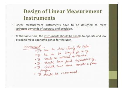
So, the design for linear measurement instrument is the linear measurement instrument have to be designed to meet stringent demands for accuracy and precision. Now, you will be able to distinguish what is accurate and precision right.
