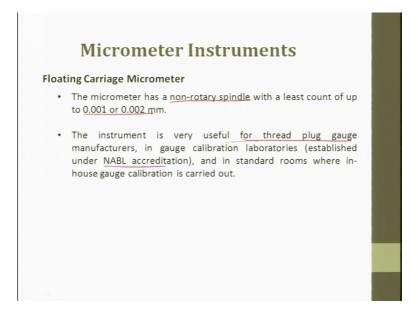
The micrometer has a non stationary spindle of a least count of 0.002; 0.2 that means, to say microns. The instrument is very useful for thread plug gauge measurement in gauge calibration laboratories which is there in NABL accreditations, which is there. So, this is a floating type. So, here you see here is a device. So, and then you can measure it. So, here you place it between the two centers and then we tight it, we lock these two and then we try to measure the deviations.
