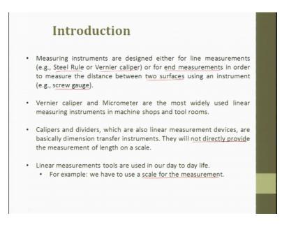
So, measuring instrument are designed either for line measurement or for end measurement. We saw earlier, how do we convert line to end an end to line we solve those things. So, when we talk about line measurement, the examples are nothing but steel ruler or Vernier caliper. In order to make sure the distance between the two surfaces using an instrument is flat.
