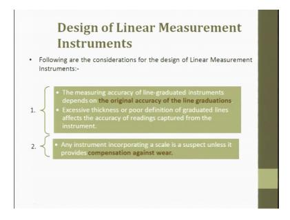
Following are the considerations for design of linear measurement instrument. The measuring accuracy of line graduated instrument depends on the original accuracy of the line graduation. Excessive thickness; so, excessive thickness or poor definition of graduating lines affects the accuracy of readings captured from the instruments, whatever I said earlier clarity. Any instrument, incorporating a scale is a suspect unless it provides compensation against wear.
