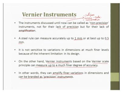
The next instrument for discussion is Vernier caliper. This instrument until now can be called as non precision instrument due to the lack of precision, but for their lack of amplification. A steel ruler can measure accurate up to 1 millimeter, at the best it can go up to 0.5 millimeter.
