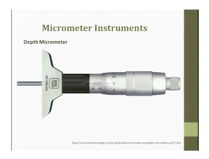
So, this is the depth micrometer. So, again same with a thimble, you have a main scale reading and you have a Vernier.
