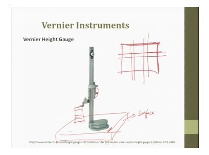
So, this is the, this is a Vernier Vernier depth gauge, this is Vernier depth gauge and in the very similar fashion you will also have Vernier height gauge ok, I have Vernier height gauge. So, here is a Vernier height gauge, this Vernier height gauge by the way can be put on a surface plate. This is a surface plate, where the reference on the surface and the flat on the base are buttered with each other, so that you do not get any angle theta value for this plane.
