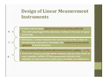
The cost is not an issue; digital display may be preferred because when you talk about second decimal and third decimal using mechanical and then screw gauge, it is always now becoming difficult. So, it is better to have a digital display and the digital display displays to the second and then third decimal to get good results and of course, today electronics are the stability of the electronics have improved a lot.
