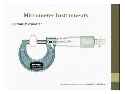
So, this is the outside micrometer. So, or people call it as screw gauge ok. So, here it is 0 to 25, this is the least count they have given. So, here ok. So, this is the main scale and this is the Vernier scale or here is that screw. So, what we do is we try to keep the component here and then we start rotating and then once it is very close and it is very tight then we start rotating this knob until we get a click sound. Moment we get a click
