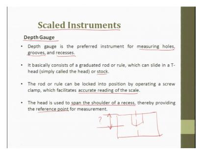
Next is scaled instruments. So, till now what we saw was we saw linear, now we are going to see scaled. First is depth gauge. Let me first to show you your depth gauge.
