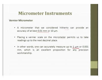
So, Vernier micrometer; so, this is outside micrometer. So, next is Vernier micrometer.
