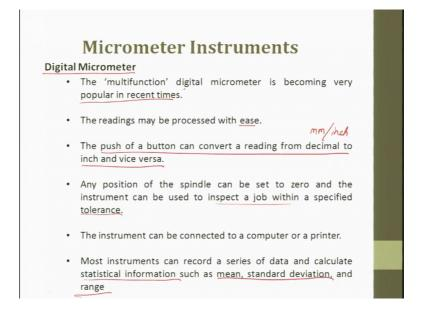
Digital micrometer is the latest which is there in order to get out of the ambiguity or measuring angle that if the principles are not followed, so, you might get to different values. So, in order to get out of it, we are nowadays using digital micrometer. A multifunctional digital micrometer is being is being very popular in the recent times. The readings are very easy to measure. The push of a button can be converted in can convert a reading from decimal to inches and vice versa.
