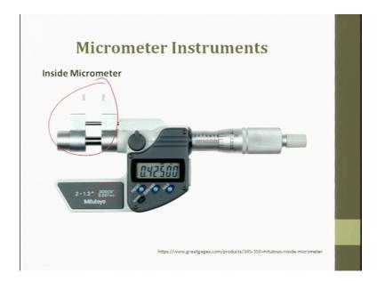
So, this is another type of inside micrometer. So, this is a slightly higher end. So, this instrument is this instrument prefers complies with Abbe's law, the Abbe's law, the Abbe's error, we will see that little later; Abbe's law and the axis of an inside micrometer is also its line of measurement
