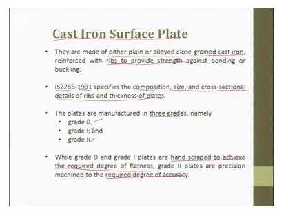
So, when we talk about cast iron surface plates, they are made of either plain or alloyed close grained cast iron, reinforced with ribs to provide strength. So, where are the ribs?
