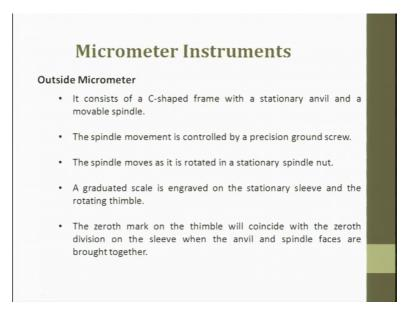
So, next we will move to outside micrometer. The outside micrometer consists of a C frame with stationary.
