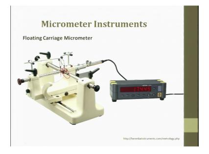
So, this is a floating carriage micrometer. So, it has a it has the carriage has a micro has a micrometer with a fixed spindle on one side, fixed spindle on one side and floating on the other. The carriage moves on a fine ground V guide ways or an antifriction guide ways to facilitate movement in the direction parallel to the axis of the plug gauge mounted between the centers.
