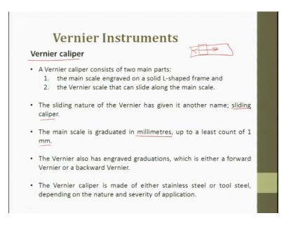
So, in a Vernier caliper, Vernier calliper consists of 2 parts. One is main scale engraved on a on a solid L shaped frame. Then you have a Vernier scale that is sliding on a main scale. So, this is the main scale, then assume that there is a block which slides on it, right; so, this is what is Vernier scale. The sliding nature of the Vernier has given it another name called as sliding caliper.
