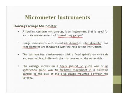
So, there is another thing which is called as floating carriage micrometer. A floating carriage micrometer is an instrument that is used for accurate measurement of thread plug gauges. So, measuring threads is also a very important parameter. So, this floating carriage micrometer is used to measure the thread plug gauge. The gauge dimensions
