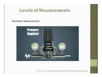
So, this is a pressure regulator. So, there is of fluid which is flowing. So, here what we do is this knob we operate to change the pressure. So, here is a pressure gauge which measures and tells you. So, this is the in and this is the out ok, this is the out. So, we do all this changes. So, this change is change in length here ok, change in pressure.
