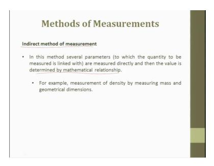
So, in indirect measurements, several parameters are measured directly and then a value is determined by mathematical relationship.
