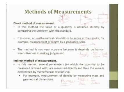
So, when you talk about methods of measurement, there are two types of measurement; one is called as direct measurement, the other one is called as indirect measurement. Direct measurement is you measure a quantity and you quickly compare it with a standard. For example, I have a vernier caliper, it has graduations, I pick up the vernier caliper, measure the shaft diameter, find out what is the error or find out what is the value.
