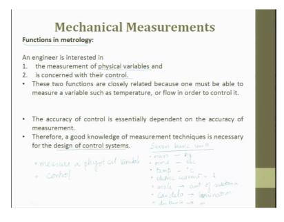
What is the function of measurement? An engineer is interested in the measurement of physical variables and is concerned with the controls also. So, these two are very important. The physical variables can be length, can be mass, can be density, can be power, can be current ok. So, all these things are physical variables.
