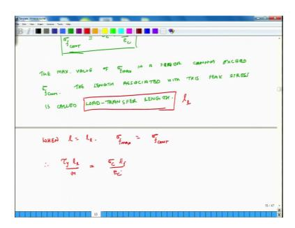
So, the maximum value the maximum value of sigma f in a fiber cannot exceed, it cannot exceed sigma f continuous. So, the length associated with this is stress; this peak stress is called load transfer length. Because we would like that are composites become as efficient as possible. So, we have to ensure that the stress in the fiber is as much as possible because fibers can take a lot of load.
