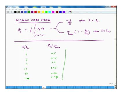
The other thing I would like to say is that there is something also known as average fiber stress. So, what is the average fiber stress basically I am trying to calculate; what is the average stress in the fiber over its length. So, this is sigma f bar and how do I calculate it? I integrate sigma f times d z from 0 to 1 which is the length of the thing and I divided by 1 this is how I calculate average of anything.
