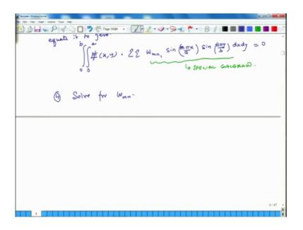
Mathematically what it means is, that I take this error and I know what this a long function is. I multiply it by a trial function; so, let that trial function be w m n 1 this is the virtual displacement and it is having the same shape as the original except that it is amplitude is w m n 1 not w m n m pi x over a sin n pi y over b. And I integrate it over the domain.
