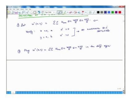
So, the second thing is we plug this w m n because we are using this special Galerkin method, and we plug it into the governing differential equation. And for making our life a little simpler actually first we will just plug it in and then we will make some simplifications. So, the second thing is this we plug this expression for w back into the governing differential equation. So, plug w not x y is equal to summation of w m n sin m pi x over a sin n pi y over b in the differential equation.
