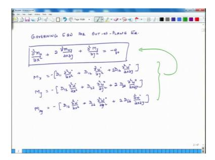
And the governing equation for out of plane equilibrium for out of plane; so, what is the governing equation? It is del 2 M x over del x square plus 2 del to M x y over del x del y plus second derivative of M y with respect to y. And that equals minus q naught so, it should be q x y, but here q x y is same is constant and it is q naught.
