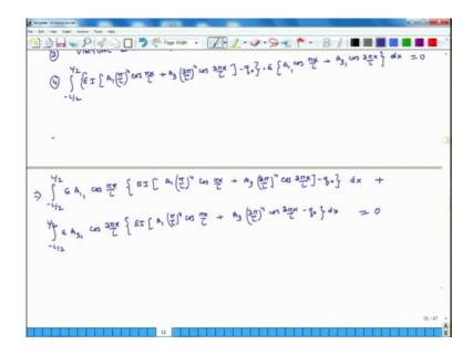
So, minus L over 2 to L over 2 EI A 1 pi over L to the power of 4 cosine pi x over L plus A 3 3 pi over L 4 cosine 3 pi x over L minus q naught. This is the error times parameter of a smallness which is epsilon times virtual displacement field A 1 cosine pi x over L plus A 3 1 cosine 3 pi x over L dx. And this is the overall virtual works. So, it has to become 0 as per the principle of virtual work.
