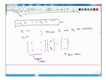
So, you will have a 2 by 2 matrix multiplied by vector A 1 A 3, and on the right side left right side you will have another matrix. So, this is called the stiffness matrix, and this is called the force vector. And A 1 and A 3 are amplitudes of the displacement component, right.
