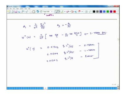
And the results are a 1 is equal to 4 over, excuse me, pi to the power of 5 q L 4 divided by EI, and A 3 is equal to a 1 by 35 negative of that result what we find out. So, w naught x is equal to 4 over pi to the power of 5 cosine pi x over L minus 1 over 35 cosine 3 pi x over L. So, this is the 2 term solution.
