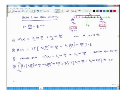
So, we will generate the solution for a beam for 2 term solution. So, if we know how to do 2 we can do 3 4 term or whatever. So, we will generate a 2 term solution, and once again the beam is simply supported on both sides. So, beam axis is at the centre. So, this is my x axis, this is my z axis and I am interested in finding out the deflections for the
