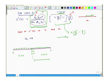
So, this is for case C I am sorry for case D. So, U nought x equals B 1 1 q a cube by 24 script A 11 divided times D 11 into 4 x over a square minus 1 times x over a ok. Now let us look at all these parameters q is positive a is positive A 11 is always positive and so, is d 11. So, this entire thing will always be positive number ok.
