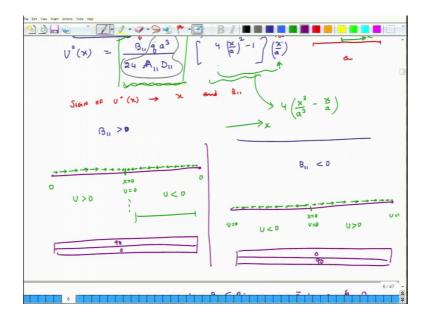
So, if this is the length of the plate at x is equal to 0, x is 0 here, U will be 0, U also U is 0 here at the boundaries because, that is how we have its prescribed the boundary conditions, but because B 11 is negative, this term in green it becomes a negative entity this is always negative this term is always negative. So, negative time negative becomes positive and what; that means, is that whenever x is positive U will be positive.
