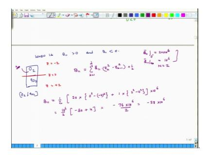
So, what is the so, when is B 11 positive and when is B 11 negative, it depends on the lamination sequence so, consider a lamination sequence 0 2 90 2. So, the lamination sequence is 0 2 90 2 which means top two layers are 0 degrees and the bottom two layers are 90 degrees and in this case this is the mid plane so, here z is equal to 0. And let us say each layer is 1 millimeter thick so, here z is equal to minus 2 and here z is equal to plus 2 ok.
