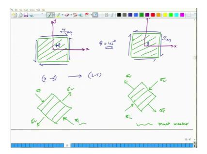
From x y plane, I have to go to LT plane. I have to compute stresses in the LT plane. Right now in the x y plane, sigma x is 0 sigma y is 0 and tau x y is not 0. But for computing failure, I have to first go to LT plane. So, I have to compute sigma L sigma T
