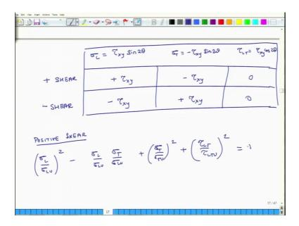
So, we make a table. So, whether it is positive or negative, we have to calculate sigma L and signal L is tau x y; sin 2 theta, sigma T is minus tau x y sin 2 theta and tau LT is tau x y cos 2 theta and we will make this table.
