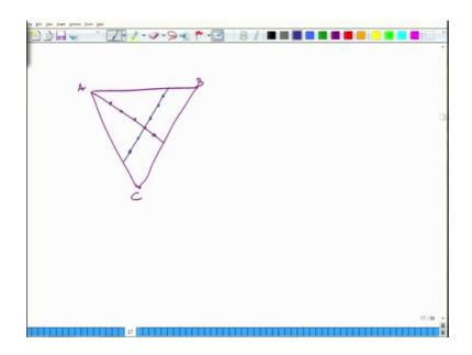
So, so, if you have this line for instance. So, all the alloy it is A, B, C; all the alloys that fall on this line will have fixed B to C ratio irrespective of composition of A. Similarly, if you have something like this and all the alloys that fall on this line will have fixed
