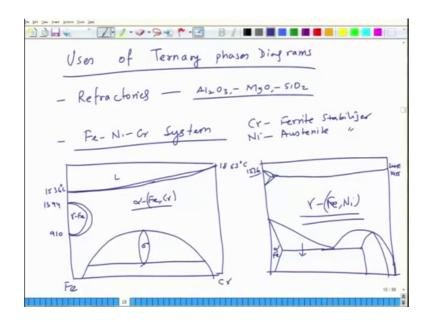
So, uses of ternary phase diagrams. So, for example: as I say refactories, so, you have you may have Al 2 O 3 M G O S I O 2 system. This is a well known system which has it is utility in lot of applications. So, if you understand the phase diagram of this composition, you can determine the compositions for which the melting point of eutectic will be minimum and then you can determine design that, will that system easily. Similarly, for iron nickel chromium system, this is the design of steels.
