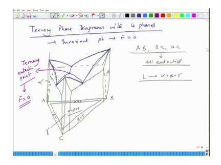
So, ternary phase diagrams with the thing about 4 phases is that you get an invariant point at which degree of freedom is equal to 0 and that is generally the you can say the eutectic point in these alloys. So, for example, your scenarios your scenario could be like this. So, I am going to draw a slightly oblique diagram just for the sake of illustration right. The first phase diagram is on the back.
