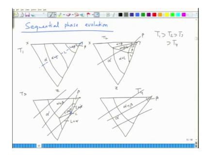
So, sequential variation phase evolution; so variation in types of phases as you go on decreasing the temperature so you may have various scenarios. So, for example, in this case one scenario could be you know used. So, it is not going to be very exact as compared to the as according to the phase diagram that is drawn, but this is just a schematic ok.
