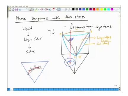
And then we also introduced, so we first initiated with phase diagrams with two phases. So, those phase diagrams basically have liquid, going to liquid plus solid and then you have solid as you go down in temperature ok. So, I mean examples of such systems could be you know isomorphous systems. Isomorphous systems where A B B C and C A all 3 of them make isomorphous phase diagrams and eventually what you obtain in the case of a ternary system is something like this. So, you have.
