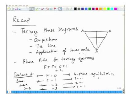
So, basically we introduced ternary phase diagrams and in those diagrams we looked at a few things like you know; how to determine the composition? What is the tie line? What is the line of fixed composition? What is the horizontal line parallel to any particular sides of the triangle?
