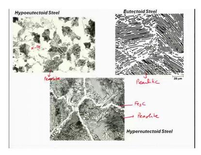
So, this is the hypoeutectoid steel on the left you can see that these are alpha Fe grains and this is what is pearlite. This is a completely pearlitic microstructure 100 percent pearlite. And this is what is hypereutectoid steel this is Fe 3 C and this is what is pearlite ok.
