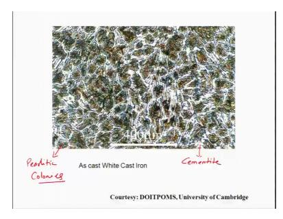
A micrograph of white cast iron is something like this. So, this is as cast white cast iron you can see the white phase here is cementite. And the gray phase is the pearlitic colonies.
