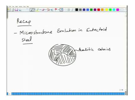
So, in the previous lecture we did we studied the microstructure evolution in eutectoid steel. Where we saw that you know you the micro structure consists of paralytic colonies and this perlite is basically a mixture of ferrite and cementite. So, next we will take up the microstructure evolution in hyper and hypo and hyper eutectoid steel.
