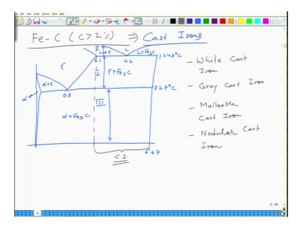
So now, let us look at F e carbon part of the phase diagram where carbon is more than 2 percent and this is called as these alloys are called as cast irons. So, now again let me draw the phase diagram of that particular part. So, you have.
