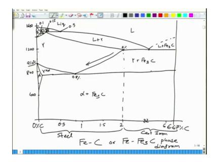
So let me draw, the iron carbon phase diagram. So, this is iron carbon or it is also called as iron cementite phase diagram. Cementite is a metastable phase so, that is why, it is normally referred as iron carbon phase diagram, because carbon is the more stable phase of the two.
