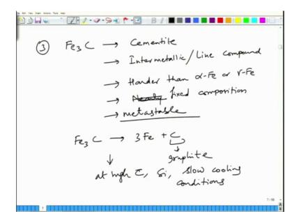
So, virtually pure iron does not consist of any carbon in it at low temperature, but whatever carbonate possesses, it is sufficient to provide it higher strength as compared to absolutely pure iron. And third phase that we have available is cementite, which is a line compound and this it is a inter metallic or line compound it is harder than alpha Fe or gamma Fe, it has nearly fixed composition.
