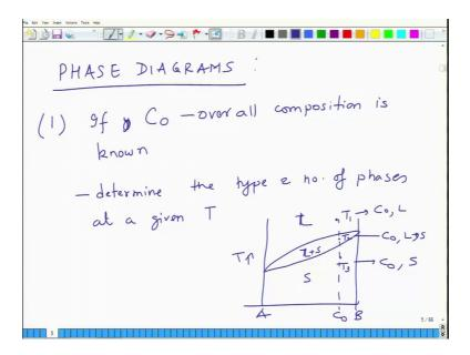
First thing that we have seen is if you know if let us say C naught, overall composition is known then you can determine the type and number of phases at a given temperature. So, this is the first utility of phase diagram. So, we can see that when you draw a phase diagram between A and B let us say you have isomorphous system.
