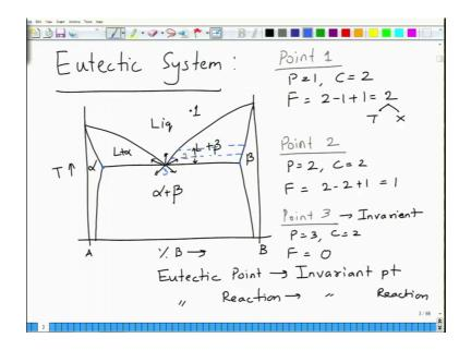
So, and this approach can also be used in peritectic in other systems. So, eutectic system is basically the phase diagram is something like. This is temperature, this is percentage B lets say and here you have liquid phase alpha, solid solution beta solid solution, two phase region. So, what you have here is basically if you look at this point for example, in this range this is 0.1, so, at 0.1.
