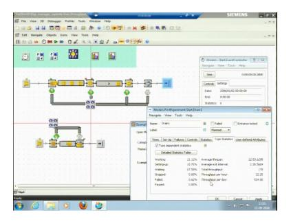
The final drain here, I can see the throughput here; What is the throughput? What is the total number of components those are manufactured in a day? This is throughput per day, if you see here this is throughput per day 534 pcs and throughput per hour just 22.25 pcs.
