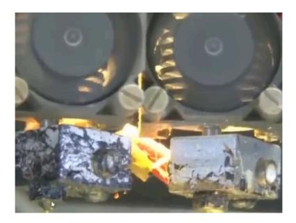
We can see that the loading of filament is properly done. Now we can see that whether the filament is coming through the nozzle or not, yes it is coming. Now this means the temperature is now maintained.
