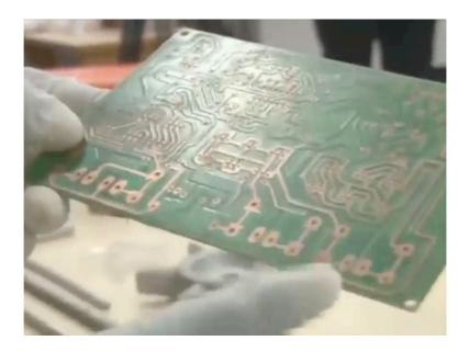
And then we have the chemical coating also to make it green coated at all and the copper tracks are there. And to prevent it from oxidation, we use green coating and green liquid is here to make it free from oxidation that is, green coating is happening.
