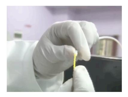
Now, we are entering the filament into the tube that is connected to the PU connector. And this tube is also very much according to the diameter of the filament, 1.75 inside diameter 1.75, plus allowance. Allowance is 0.11 0.85 mm in a dia.
