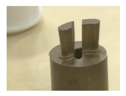
So, there is one more job of brass; this profile is called as aerodynamic profile. So, our students at IIT Kanpur of working on this high pressure air, this specific component is used to there. So, this kind of job also is carried out with the subtractive method of machining only, with milling machine.
