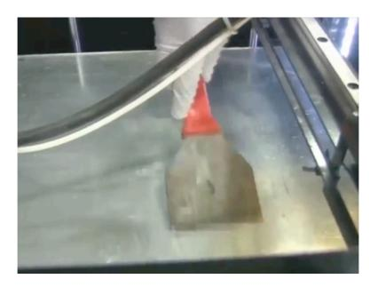
So, some of the liquid cleaner is sprayed and it is cleaned with the help of spatula. So, the whole machine header is actually glass, so we have to be careful. So, what is this white milky material? White milky material it is nothing, but we have used fevistick that is the adhesive material, this Fevistick.
