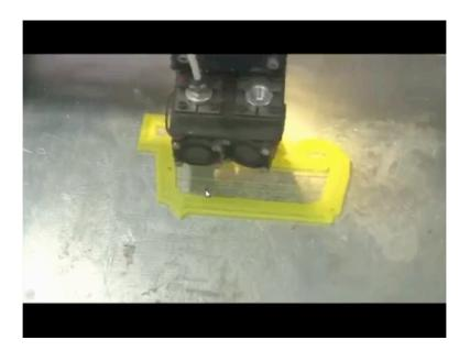
In that case, we will have a support any modern materials you know now this is happening this first layer was brimmed. And after first layer, the other layer, the second layer is now being manufactured. But it is preparing support; you can see it is preparing support here because it was an angle in the component.
