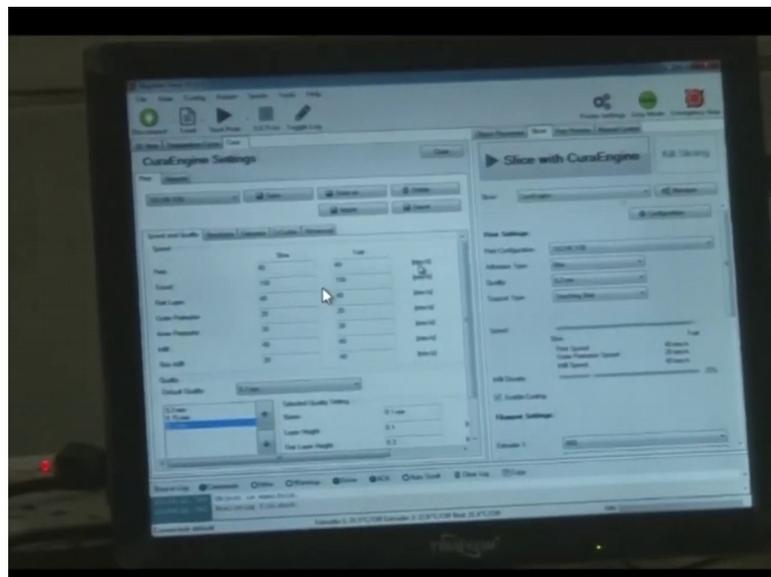
So, the travel speed of the nozzle has to be dazed. So, it is kept slow and fast it is same that is the fixed speed is 40 millimeters per second. For printing it is 40 and 40 for travel. Travel means, when it is not printing, when it is not productive it is moving just ideally from one place to another, if the speed is high it is 150 and 150. 150 means both 150 slow and 150 fast means the speed is fixed to 150 millimeters per second.
