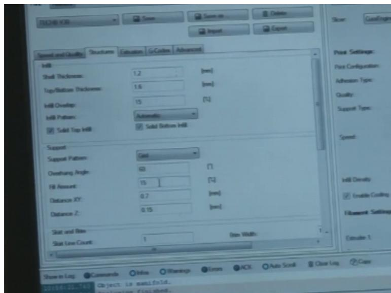
So, over an angle is 60 degree here. So, over an angle here will be for the machinery, for this machinery. If, we are going to deposit, I will better say deposited print or manufacture the job. If it is solid, there is no issue at all. If, it is a conical shape and angle is up to 60 degree.
