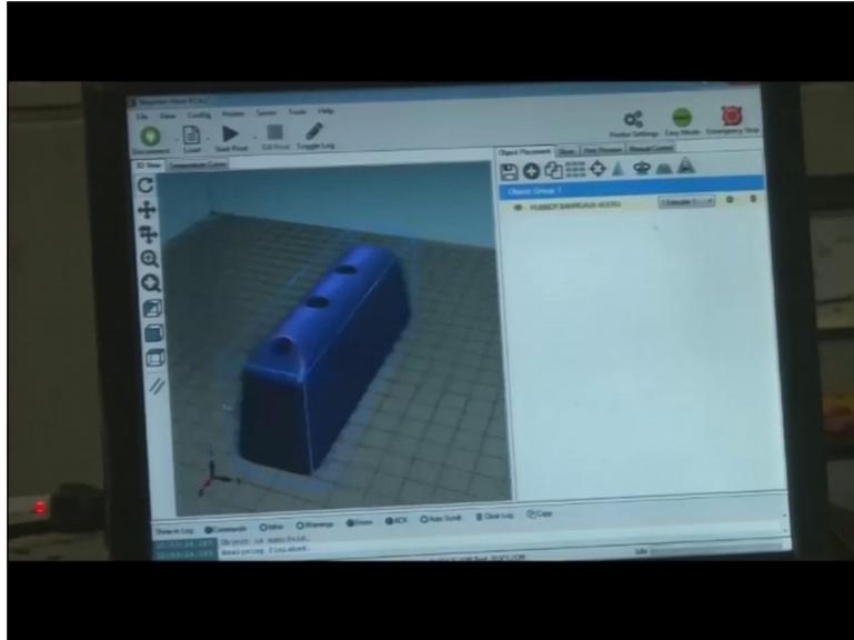
So, we will click here. So, yes when we click here this job is there here on the envelop. What is envelop? Envelop is this where we are going to manufacture this thing. So, this is 1 cubic feet, that is 1 feet by 1 feet by 1 feet, the envelop size is this one. So, this area is 1 feet by 1 feet, I can say that on the area of 1 feet by 1 feet or 1 square feet this object would be manufactured, ok.
