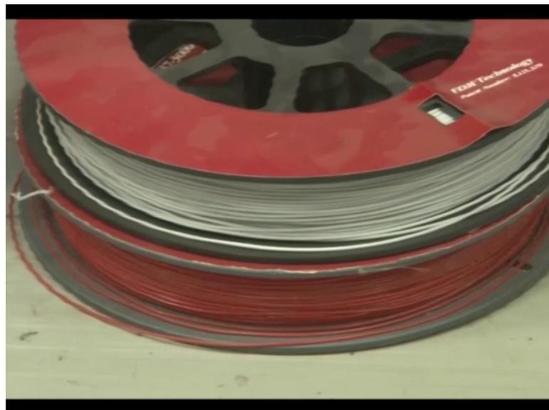
What is filament? Filament is the raw material that we are using for printing, like I mentioned ABS or PLA that is there in the filament form, this is the raw material, this is filament. So, this is white color ABS filament, this is rolled on spool.
