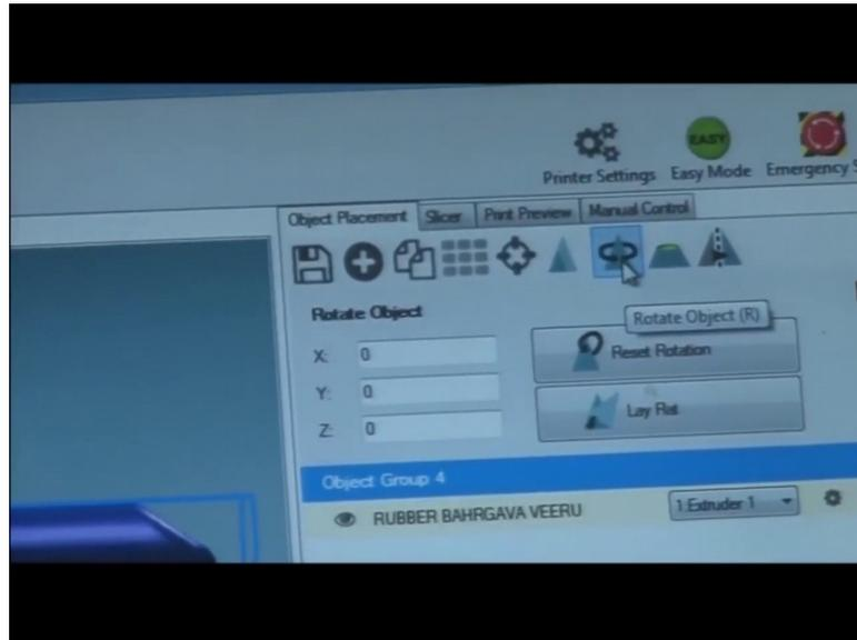
So, next I can do here is rotate object. Sometime,s like I discussed like we have discussed as the placement of the object or the alignment of the object in is very important in deciding the support material that is used, what is the amount of support material that is used.
