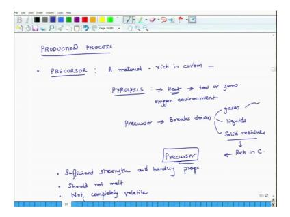
How are graphite fibers produced? So, to produce a graphite fiber you need some raw material, you need some raw material the raw material used for graphite fiber is called a precursor, precursor, that is the raw material. And what is; if we have to define what is precursor, it is a material which is rich in carbon because if you have to produce carbon fibers you need to lot of a carbon. So, it should be rich in carbon and this material when
