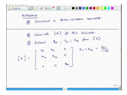
So, our approach A first thing is, construct a Quasi-Isotropic Laminate. We construct a Quasi-Isotropic Laminate, and the more the number of layers we put in this Quasi-Isotropic Laminate the better it will be because fibers will be spread more or more
