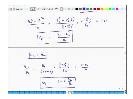
I can calculate ER for the randomly oriented mat by this relation, ok. So, if for a Quasi-Isotropic Laminate I know A 11, A 12 then, I can say that A 11 square minus A 12 square divided by A 11 will be the Young's modulus of a randomly oriented mat, ok. Next we will see how does G work out. So, GR is equal to A 66 that is direct because, thickness we have assumed as unity ok.
