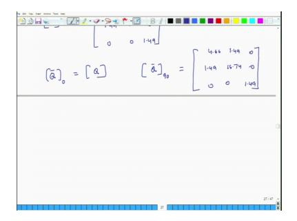
So, Q bar for 0 degree is same as Q matrix, ok; for 90 degrees thing, Q bar for 90 degree it is we just replace 16.74 by 4.66 and vice versa. So, it is this 4.66, 1.49, 16.74, 1.49, 0, 0, 0, 0 and 1.49 ok. And for 45 degrees we actually use the relations which we have explained in the class.
