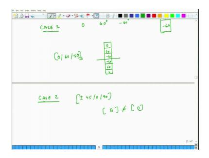
So, you can have 0, 60, minus 60, minus 60, 60, 0. So, this is essentially 0, 60, minus 60, symmetric and in this case B will be also 0 and it will still be quasi isotropic because A matrix only depends on the thicknesses A matrix only depends on thicknesses. So, the same sequence is being repeated. So, the quasi isotropic will be retained.
