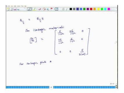
And then what about the A matrix? So, the A matrix elements can be defined as Q ij times its just single layer because its one single material, so thickness of the plate, right.
