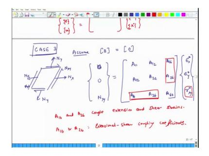
Let us look at some more cases. So, there is a third case ok, third case. And here we look at the a matrix in detail. So, we assume that we have designed the plate such that it is B 0, you have designed such that it is B 0 and we are loading the plate only in using N. So, the plate is experienced in N x and y and maybe also N xy, ok.
