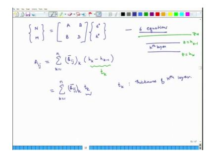
So, overall the relationship which we had developed was there is a n vector and there are moment resultant. So, they are related to this 6 by 6 matrix which is made up of A B and D sub matrices times midplane strains and midplane curvatures.
