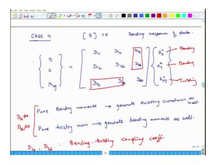
So, this is a bending curvature this is a bending curvature and this is a twisting curvature, is the twisting curvature. Now, consider a situation where I apply only M x, and I do not apply M y and M xy, so M y and M xy are 0. In that case if these terms are nonzero D 16 and D 26 then pure bending moments. So, M x is a purely bending moment they generate twisting curvatures as well ok, because D 16 and D 26 is not 0. Similarly, if I apply a
