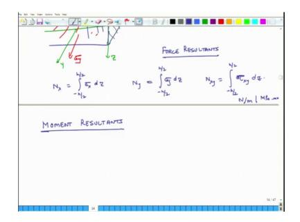
So, similarly we define other quantities. So, N x is equal to integral of minus h over 2 to h over 2 sigma x d z similarly N y. So, what is N y? In this direction this is sigma y. So, if I integrate sigma y on this entire surface and then I use it on upper unit length basis then then I get N y, so that is equal to sigma y d z.
