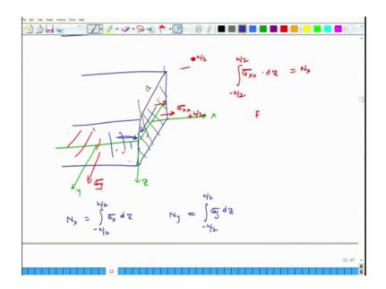
So, we define resultant forces as N's and moments as M's and these are resultant forces and moments per unit length they are not their units are not Newtons and Newton meter because they are per unit length ok. So, we will actually define that. So, first we will explain the concept.
