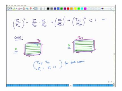
So, it is sigma L divided by sigma L u prime minus sigma L divided by sigma L u times sigma T divided by sigma L u plus sigma T divided by sigma T u whole square plus tau
