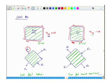
So, it does not matter, next look at case B and this is where you will see the difference case B. So, here also we have oh I am sorry it is not case B case 2 and here we have 2 situations in the first situation we have fibres oriented at 45 degrees and in other situation also fibres are oriented at 45 degrees, in both the situations fibres are oriented at 45 degrees.
