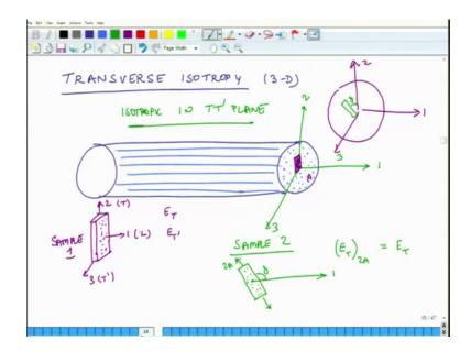
The second case is we will talk about is transverse isotropy, transverse isotropy. So, first case which we had discussed was fully anisotropic then we simplified it and especially
