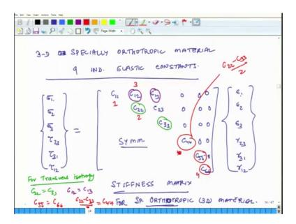
So, a 3 dimensionally especially orthotropic solid will have 9 independent elastic constants. So, a 3-D specially orthotropic material, 3-D specially orthotropic material it will have 9 independent elastic constants, ok.
