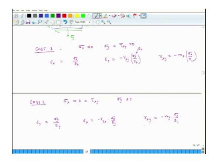
So, again we will have four different cases case one. In the first case, we have only sigma x. So, sigma x is not equal to 0 sigma y and tau x y are 0. Now, this is the case of general or orthotropy. So, when I am pulling the material it will not only exhibit extensional strains, but it will also exhibit shear strains. So, we will write down the relationship between stresses and strains.
