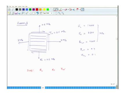
So, example; so, the problem is that we have a lamina fibers are oriented in this direction and I am loading it in such a way that sigma L is equal to 3 MPa. It also has transverse load such that the transverse stress sigma T is equal to 0.5 MPa and then there is a shear stress and the shear stress equals 3.5 MPa.
