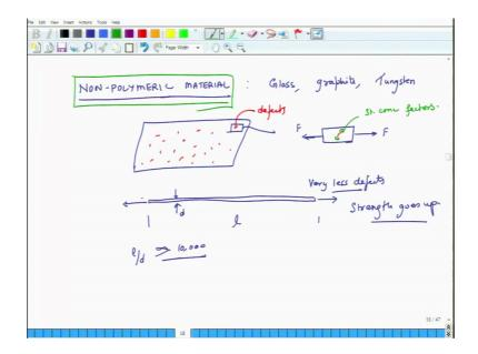
So, we will consider two types of materials the first is non polymeric materials, non polymeric materials examples would be glass graphite, we also saw the example of tungsten and so on and so forth. Now if you look at the bulk material and you make a cross section of it and you look at it very closely what you will find is that in the bulk material there are very small flaws defects.
