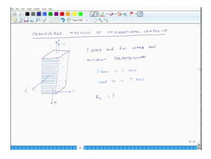
So, what do we mean by transverse modulus what we imply is. So, let us say this is a sample of composite material and here the load is in the transverse direction what does that mean. So, let us say I am still loading it in this direction, but the fibers are not aligned with the direction of the load rather fibers are at ninety degrees to the load.
