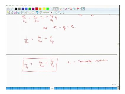
So, but sigma m equals sigma f equals sigma c. So, what I can write it as 1 over E c is equal to V m over E m plus V f over E f.
