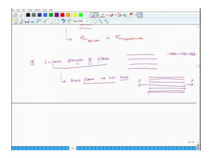
But for glass fibers, this may not be true there is a significant statistical variation you take twenty different fibers there are lot of imperfections in glass fibers especially because they are they have high abrasion and that that damages the fibers.
