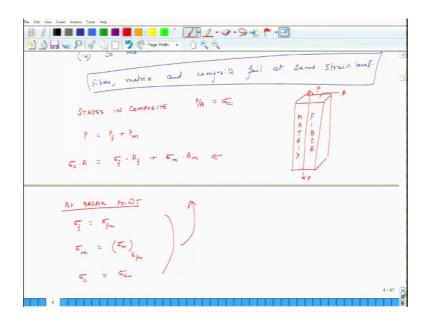
So, here this is my fiber and let us say this is my matrix and I am pulling it with a load P I am pulling it with a load P. So, what is the stress in composite? Stress in composite is P by A. So, that is equal to sigma c right, sigma c.
