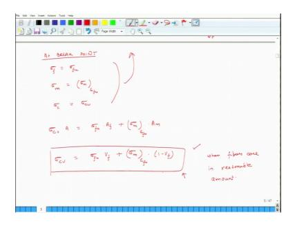
So, I get sigma c u times A is equal to sigma f u times A f plus sigma m evaluated at breaking strain of the fiber times A m.
