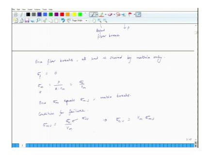
Once fiber breaks, all the load is being shared by matrix only all load is shared by matrix all the load is shared by the matrix. So, in that case sigma f the stress and fiber is what is 0 and the stress in matrix is what? What is the stress in matrix? Well total load is external load is force and what is the area of matrix area times V m right this is the area of the matrix.
