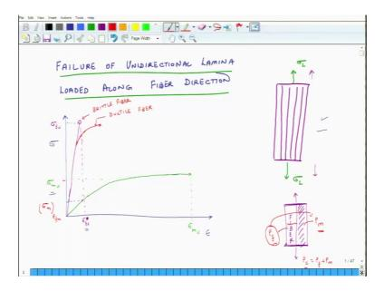
So, what we will discuss is failure of unidirectional lamina loaded along fiber direction. So, what does that mean what it means is that suppose I have a unidirectional composite and the fibers are aligned along the length of the composite and suppose I apply an external load sigma L why do I call it sigma L because it is in the longitudinal direction we had defined longitudinal transverse and transverse prime directions in the last week.
