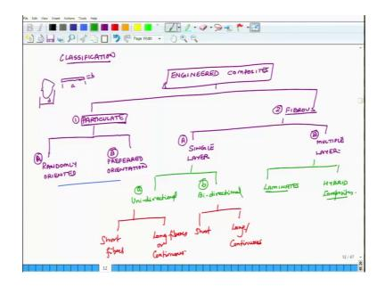
And when we are doing this, we are only going to address engineered or engineering composites. We are not going to worry about naturally a composite such as wood or bone or granite and things like that. So, will talk about we are going to do this classification in context of manmade composites.
