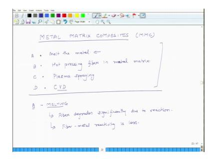
Metal matrix composites or MMCs. So, in metal matrix composites we all know that metals melt at higher temperatures. So, we have to use high temperatures for processing metal matrix composites.
