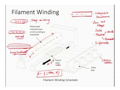
So, this is a schematic which talks about filament winding. Now what you have here, are a large number of fiber rolls and this entire set is known as a creel. So, you have a creel in, which you have different roles of fibers.
