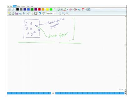
So, these are all pellet us and they are surrounded by matrix and this is what. So, these are all pellet us they are surrounded by matrix they are separate. So, this matrix is thermoplastic matrix. So, it is a thermoplastic polymer and these short fibers. So, this is my short fiber this short fiber is a lot of times; it may be glass sometimes may be it may be have some other fibers. So, each pellet has some short fibers in it bound by matrix.
