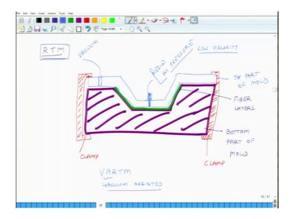
So, a limitation of the vacuum bag molding or bag molding processes is that the fibers when you apply a lot of pressure, they tend to dislodge from their original position and there is a chance that the orientation of the fibers. In the system especially if you use pressure external pressure may not be same as what you intended, because the as you apply external pressure. The fluid in the thing flows at a higher velocity with high pressure and it tends to change the orientation of the fibers.
