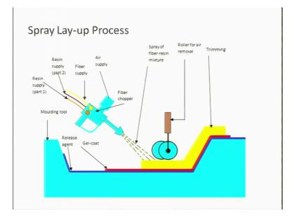
This is the picture which is a schematic for spray layup process. So, this blue thing is your molding tool on top of the molding tool as we had discussed is the release agent which ensures removal of the part from the mold, to provide finish you have this red layer which is a gel coat. And then through this tool which has 2 nozzles or in this case at least there are everything is coming from the same hole.
