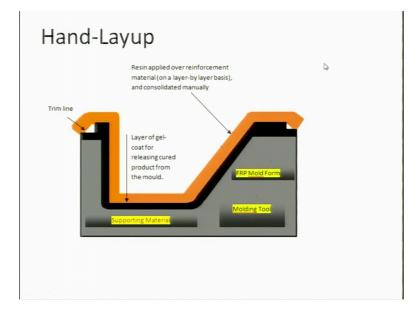
So, this picture is about the hand layer process. So, what do we see here? So, here we have a mold and you see that the mold is. So, suppose you want to make the material which is indicated in.
