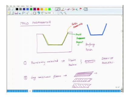
Mold preparation this is a very important stage in hand layup process. So, suppose I want to make a shape suppose this is the shape I want. So, what do I do? I make a mold which will be which will have a shape similar to it. So, this is the first step. I make a mold. And this could be made up of something inexpensive.
