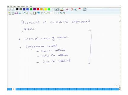
So, selection of production composite fabrication process, which type of process should we choose? There are several processes and we have to think as to what is the right type of process. So, when we do this, we have to be aware of 2 or 3 very important parameters, the first thing is that we should have an understanding about the chemical nature of matrix.
