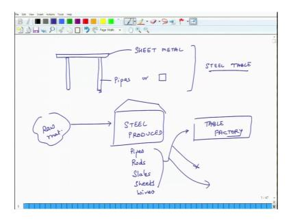
So, the table which has made up of steel would consist of what? So, I want to make a table, so it will have a top and it will have some legs basically. So, what do I do? To make the top typically a lot of these tops are made from sheet metals and the legs, so this is the leg and typically these legs are made up of pipes or maybe some other cross sections maybe some rectangular cross sections. So, this is how a regular steel table is configured.
