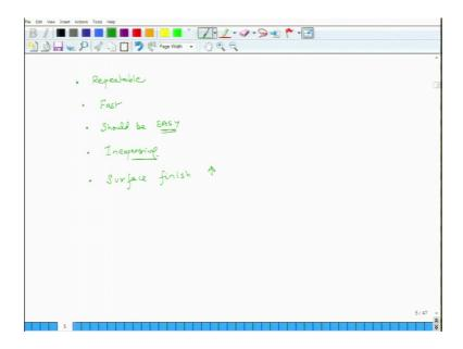
The fabrication process to be repeatable, so each time we make the same composite structure with same chemical formulation, same percentage of fibers, same matrix, we should get the same product with same mechanical properties and other properties, so it should be a repeatable process.
