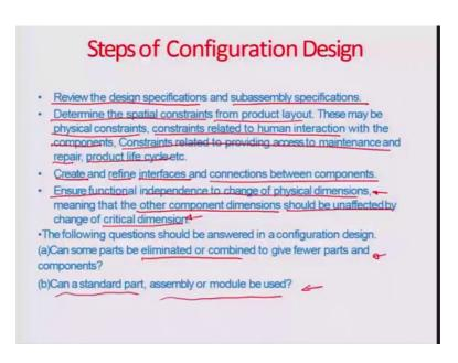
So, the in summary the steps of configuration design are to sort of review the design specifications and the subassembly specifications. Determine what are the spatial constraints particularly from the product layout these may be physical constraints, this may be constraints related to human interaction with the components, or constraints
