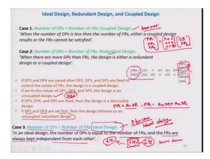
Now, what is the ideal design, redundant design and coupled design, again you can distinguish your design in an another form that is for case one if number of design parameter is less than number of functional requirements that is called coupled design that bad design bad one.
