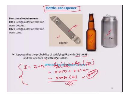
Now, I am giving you one real example that is the bottle can opener and we are going to calculate information matrix for that bottle can opener this is the bottle can opener using this you can open your bottle beverage bottle as well as your aluminium can. So, it has a more than two functionalities, so it is available to open both of these. So, what are the functional requirement for this problem design a device that can open bottles and design a device that can open cans ok.
