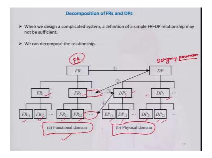
Now decomposition of functional requirements and parameters, so in an ideal condition functional requirements and parameters are a very few in numbers, but in actual condition there are a lot of requirement functional requirements involved there to in a fabrication of one product.
