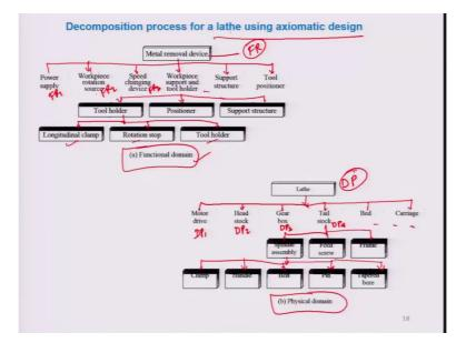
Decomposition process for a lathe using an axiomatic design. So, for lathe what you have to do for lathe what is the function of lathe it is a metal removal machine ok. So, for material removal device what are the functional requirements you have a functional requirement.
