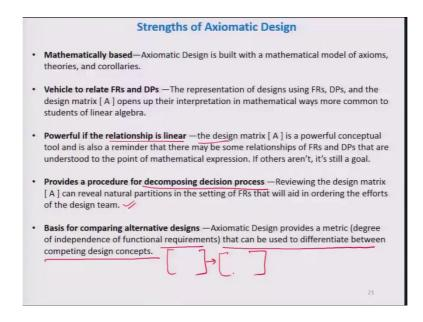
Now, what are the strengths of the axiomatic design. So, first you can there are variety of benefits are available for axiomatic design. So, what are the strength that first one is mathematically based, second one is vehicle to related functional requirements and designing parameters third one is the powerful if the relationship is linear.
