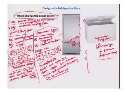
Now, I am taking giving you an another example design of a refrigerator door, here there is two kind of refrigerator is available here gate will open like this way and this case gate will open like this way. So, that is the horizontal hung door and it is vertically hung door.
