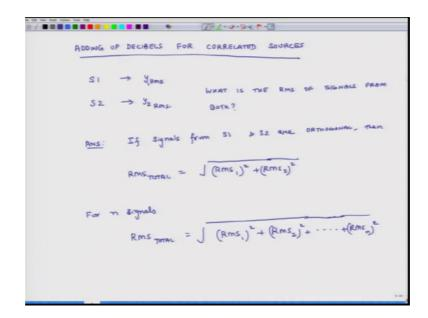
So adding up decibels for correlated sources, this is our theme. So, before we do that, we should also know how to add up, how to figure out the RMS value of two correlated signals. So, what do we do, by mean by that. So, suppose there are two signals S 1 and S 2 and the RMS of this signal is y y 1 RMS, and the RMS of the signal is y 2 RMS, then the question is, what is the RMS of signal from both.
