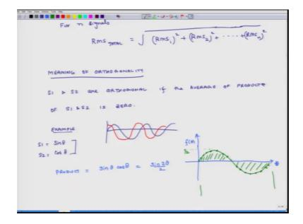
So, at least in context of today's lecture what does. So, two signals S 1 and S 2 are orthogonal, if the average of products product of S 1 and S 2 is 0. So, two signals are mutually orthogonal, at least in context of this discussion if. So, how do I figured whether the signals are orthogonal or not. Take two signals, I multiply them, I plot them on a graph and see whether the average of that gas is 0 or not example. So, example could be sin theta and cosine theta ok.
