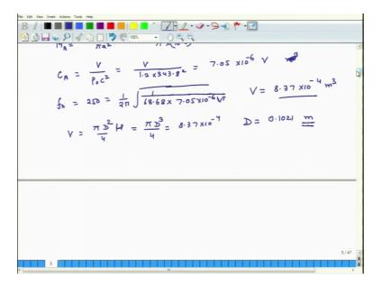
So, now I know v and I know that v equals pi times D square times height divided by 4 equals because D equals H. So, it is pi D cube divided by 4 and that equals 8.37 into 10 to the power of minus 4. So, solving for D, I get D equals 0.1021 meters ok.
