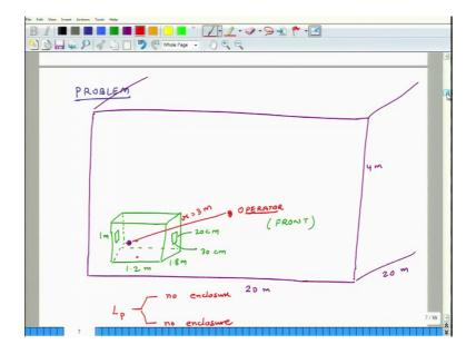
So, here is the problem. So, what we have is a machine, so its emitting some sound and it is in a large room. So, let us keep the machine here and it is in a large room something like this and the size of the room is 20 meters by 20 meters by 4 meters. So, all the dimensions are in meters.
