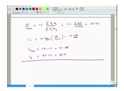
So, insertion loss is 10 log 10 W by W out and that equals 17 dB and L W out equals. So, insertion loss is seventeen decibels without the window the sound pressure level be calculated was 102 decibels. So, I just subtract 17 from there. So, this is equal to 114 minus 17 is equal to 97 dB and L p equals 97 minus 17 that is equal to 95.9.
