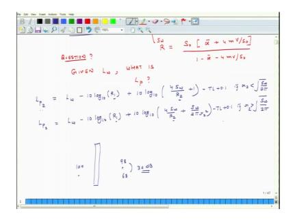
Suppose I have a wall and here it is 100 decibels, suppose, there was no wall suppose, there was no wall and here it was 100 decibels and at this point, it was 98 decibels in absence of wall, then as sound travels from here to hear it falls by 2 disable, right, suppose I introduce a wall and then all of a sudden it becomes 68 which means that the wall is causing a loss of transmission of how much thirty decibels of sound.
