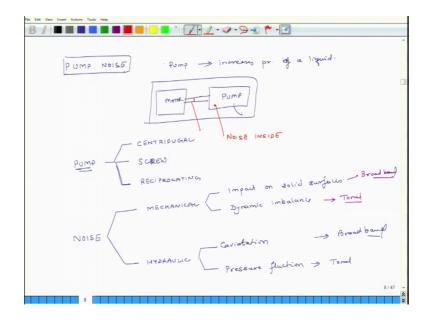
Now, once again what does a pump do? Pump it increases the pressure of a liquid and typically a pump has two parts, you have a motor which converts electricity into mechanical energy and this shaft it actually drives the pump. So, this is the pump this is the motor and this entire thing is also lot of times it is referred to as the pump.
