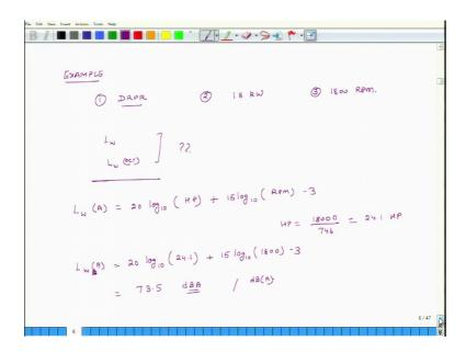
So, we will do an example on noise you are getting from a motor. So, let us say we have a motor and it is of DRPR type, DRPR that is drip prof motor. The second thing which is given is that the vertex of the motor or the horsepower of the motor. So, we are told that it is having its power is 18 kilowatts and it runs at 1800 RPM. So, with these data we are supposed to estimate L w and then L w for each octave band these are the things which we are suppose to compute.
