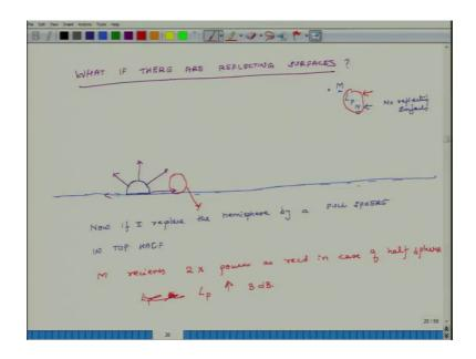
But because it is going through the center of the sphere it does not have any influence on the reading of the microphone which also means that instead if I have a universe which has a top half and a bottom half plane I do not need a whole sphere to produce the same sound pressure level, rather I just need a half sphere right. I only need half of the sphere to produce L P N, because the lower half is not being utilized agreed.
