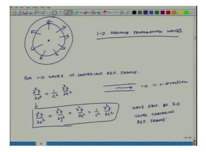
So, suppose you have a very small source of sound and the source of sound is such that it is producing sound of equal intensity in all directions and also the medium in which sound is propagating is homogeneous. So, it is not changing from point to point in a radial way. So, what will happen is that, sound waves will spread out uniformly in all directions in a radial fashion. So, they will just keep on spreading out in all directions in a radial fashion.
