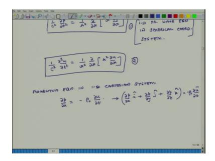
So, this is equal to 1 over r square del over del r, r square del p over del r this is what it based on to. So, this is the 1-D pressure wave equation in what? In spherical coordinate system and this equation is valid when is it valid if all the sound is coming from a point and it is spreading out in all the directions uniformly. If it is not uniform spread of sound then we have to use more general operator.
